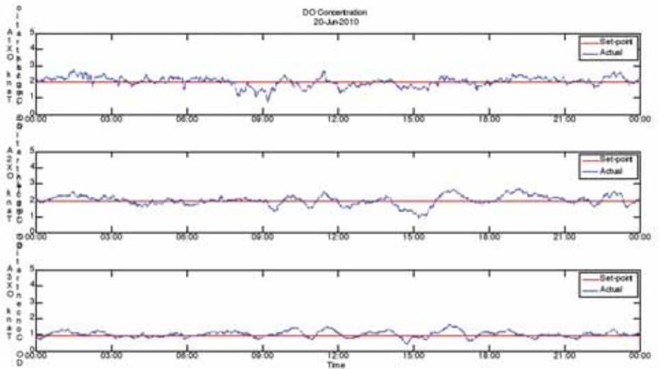
Figure 7. Dissolved Oxygen of Plant Under Automatic Control
