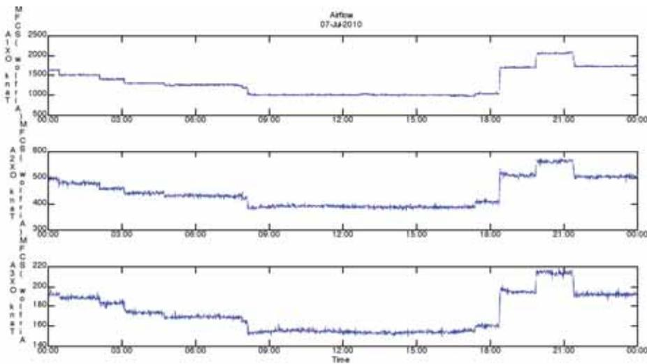
Figure 3. Airflow Profile of Plant Under Manual Control
