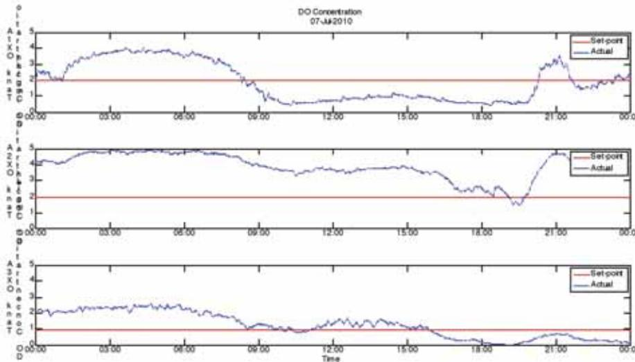
Figure 4. Dissolved Oxygen Profile of Plant Under Manual Control
