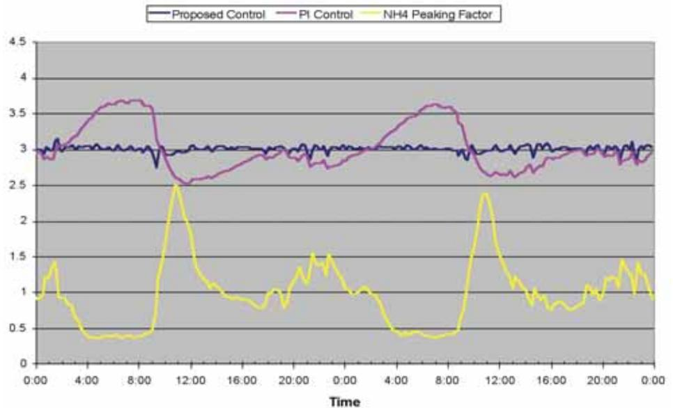
Figure 2. Proportional-Integral Control vs. Proposed Dissolved Oxygen Control Simulation
