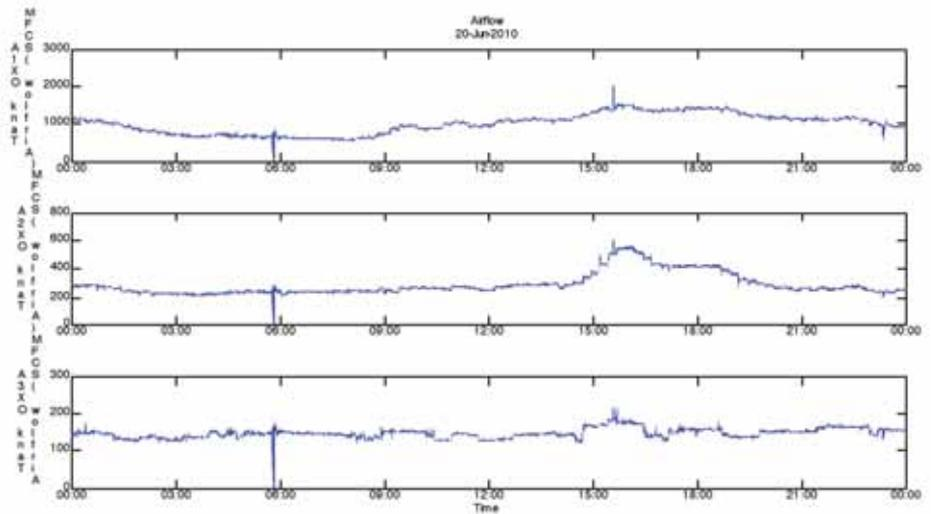
Figure 6. Airflow Profile of Plant Under Automatic Control
