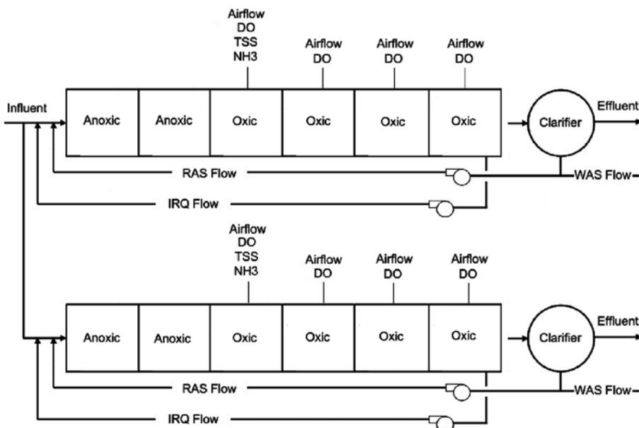
Figure 1. Process Flow Diagram of Poinciana Water Reclamation Facility No. 2
